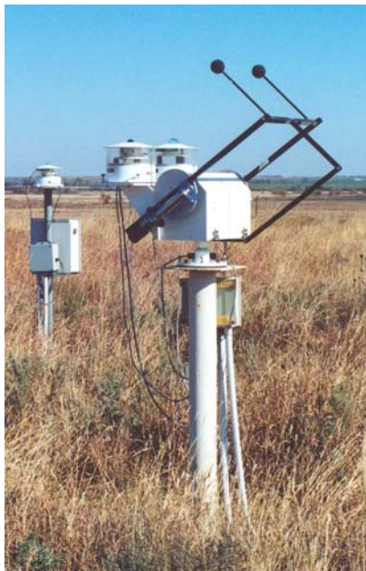
Figure 2. Unshaded pyranometer (Left) for GH measurement, shaded pyranometer and pyrgeometer (on solar tracker horizontal platform) for DIFF and downwelling longwave (infrared – for atmospheric science study), and pyrhelioscope (on side of solar tracker) for DNI measurements at the DOE/ARM Southern Great Plains station near Lamont, Oklahoma.
